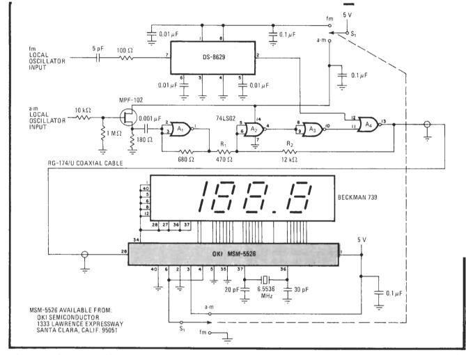
**I-f compensation.** MSI and LSI chips reduce cost and complexity of display for a-m/fm radio. MSM-5526 counter has circuitry for subtracting receiver's i-f frequency (see table) from radio's local oscillator input so that the true channel frequency may be displayed.
